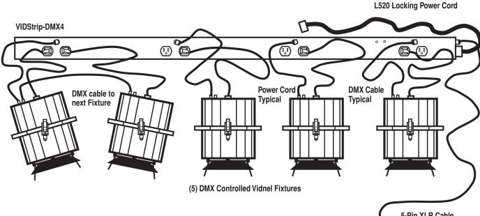
This power strip provides (8) Power outlets and (4) DMX output circuits in addition to DMX in and out pass through conveniently mounted in your grid. It is designed with opto-isolator surge protector for the (4) DMX fixture circuits and has indicator lights for power and DMX. The 20 amp unit has L520 locking plugs for power in and out.
